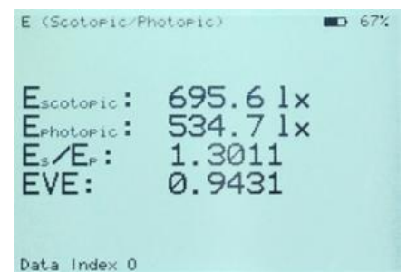
Ratio of the scotopic and photopic illuminance with the EVE factor as per IES TM-24-13
